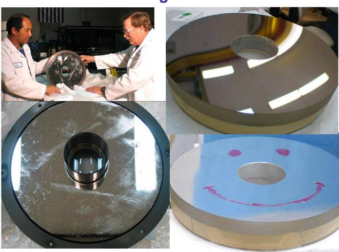
Here is a 12", 305 mm protected aluminum mirror. It was cleaned with Spray First Contact and then protected from recontamination with a coating of clear First Contact and a Red First Contact Happy Face!
